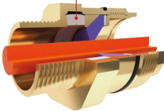
Figure 1 - When a smaller diameter cable is installed the inner compensator operates to a lesser extent.
