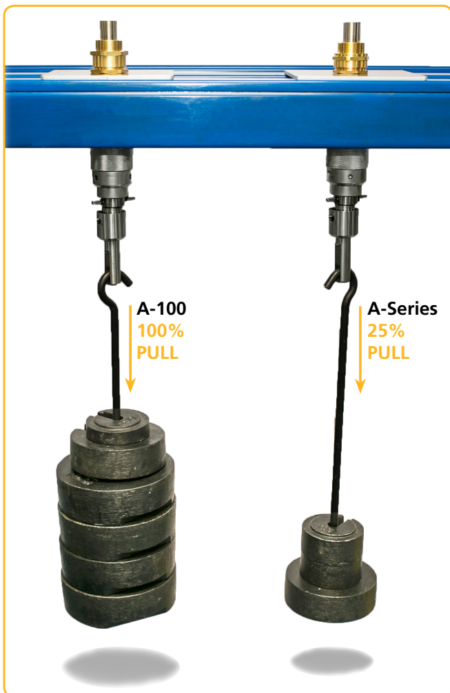
Image showing A2F100 and A2F explosive atmosphere cable glands from the A-100 and standard A series during cable anchorage test.
